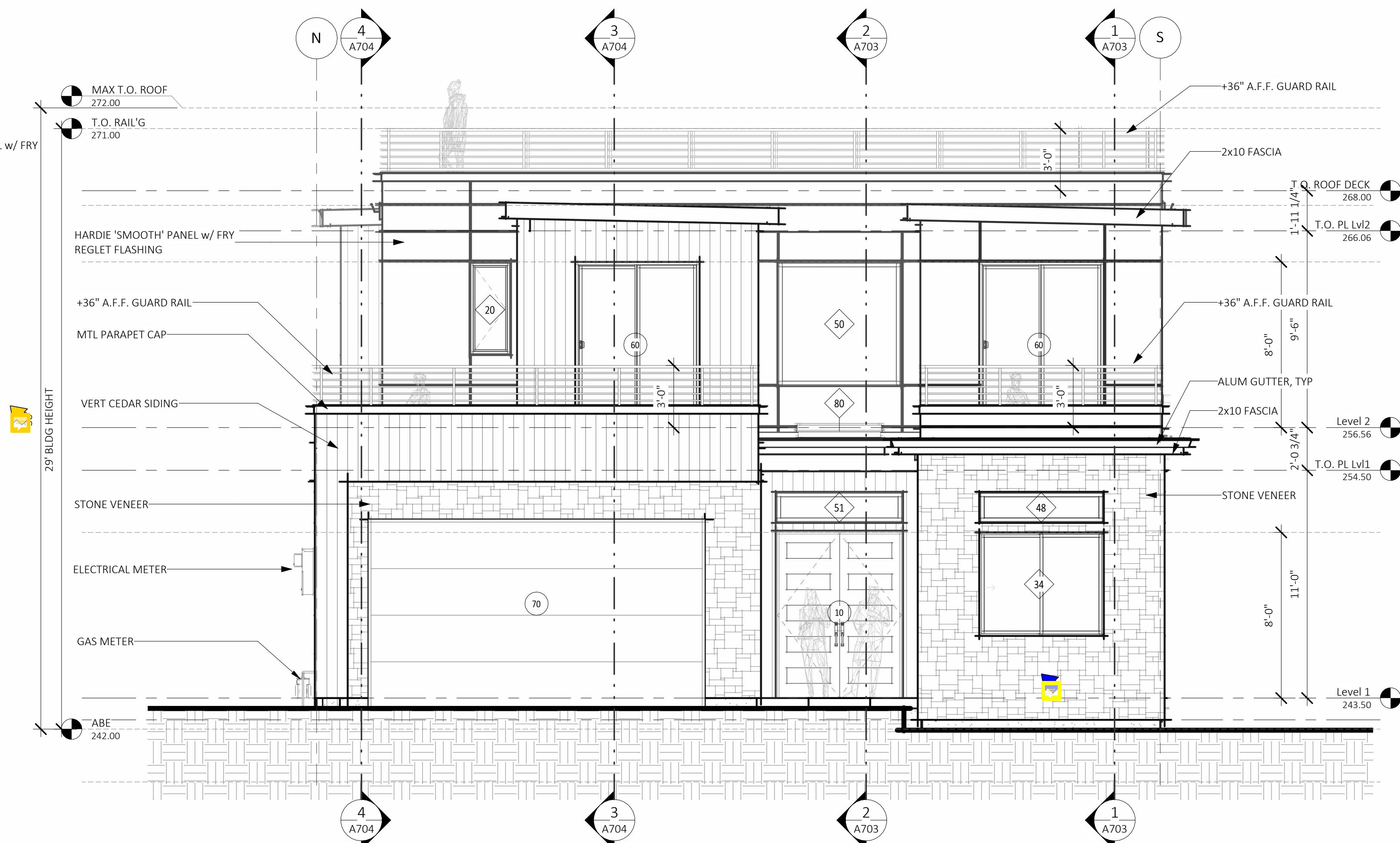
1 WEST ELEVATION SCALE: 1/4" = 1'-0"
